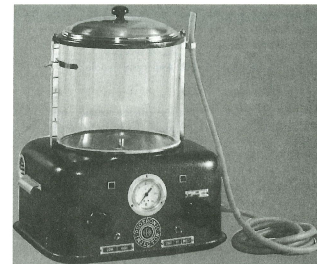
Figure 4-18. Centrifugal embalming machine. These machines are available with or without pulsation.
