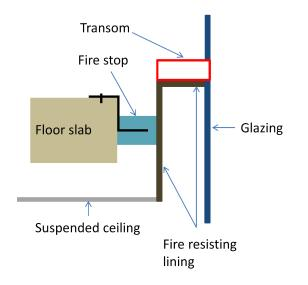
Figure B2 – Fire stopping details – storey height glazing
