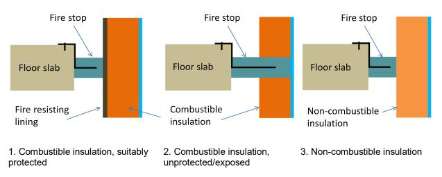
Figure B1 – Fire stopping details – spandrel zones
