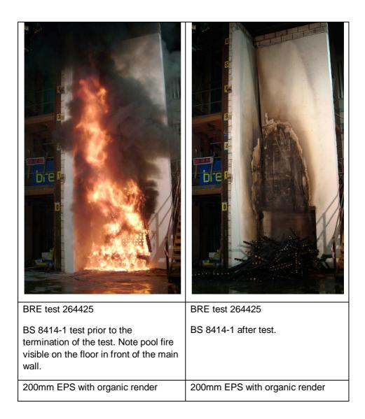
Figure 8 Photos taken for test on EPS system with organic render to BS 8414-1
