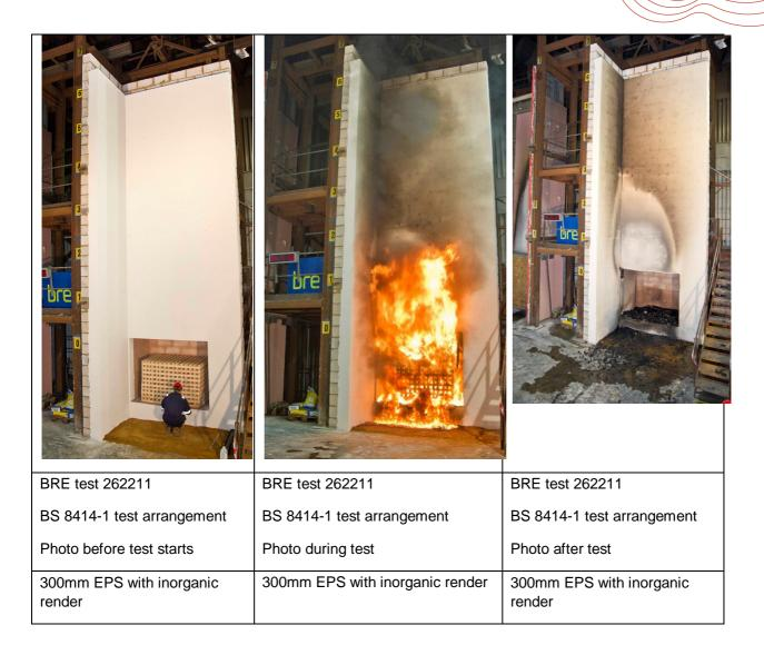
Figure 7 Photos taken for test on EPS system with inorganic render to BS 8414-1
