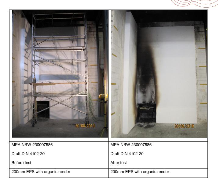
Table 9 Photos taken before and after test on EPS with organic render to draft DIN 4102-20
