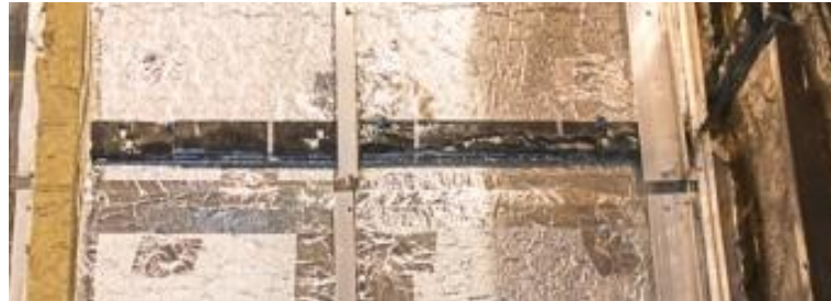
Figure 32. Zoomed view of partially activated horizontal cavity barrier at an approximate height of 2400mm above the combustion chamber, on the wing wall.
