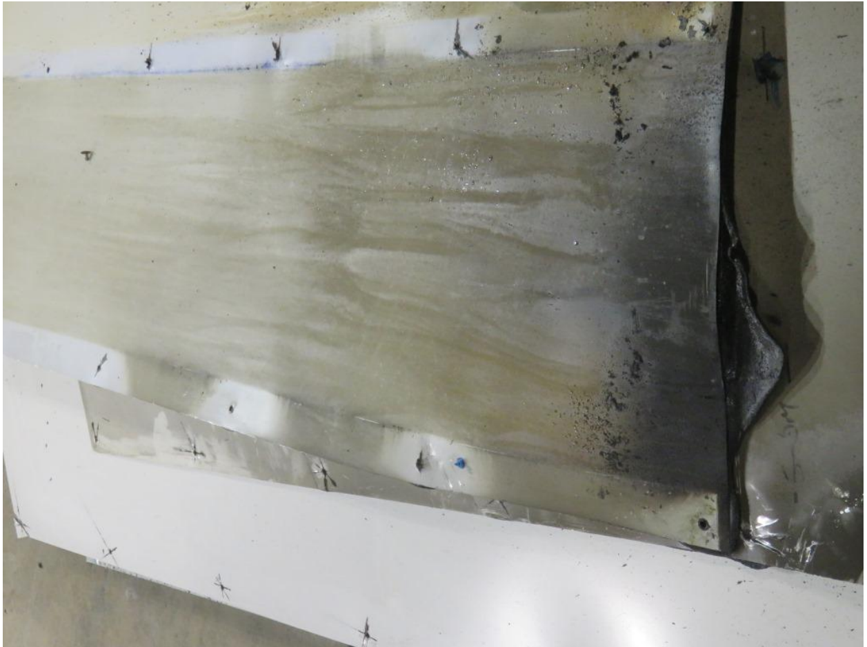
Figure 26. Rear side of panel 3C (approximately 4600mm above the top of the combustion chamber) showing re-solidified PE core material.
