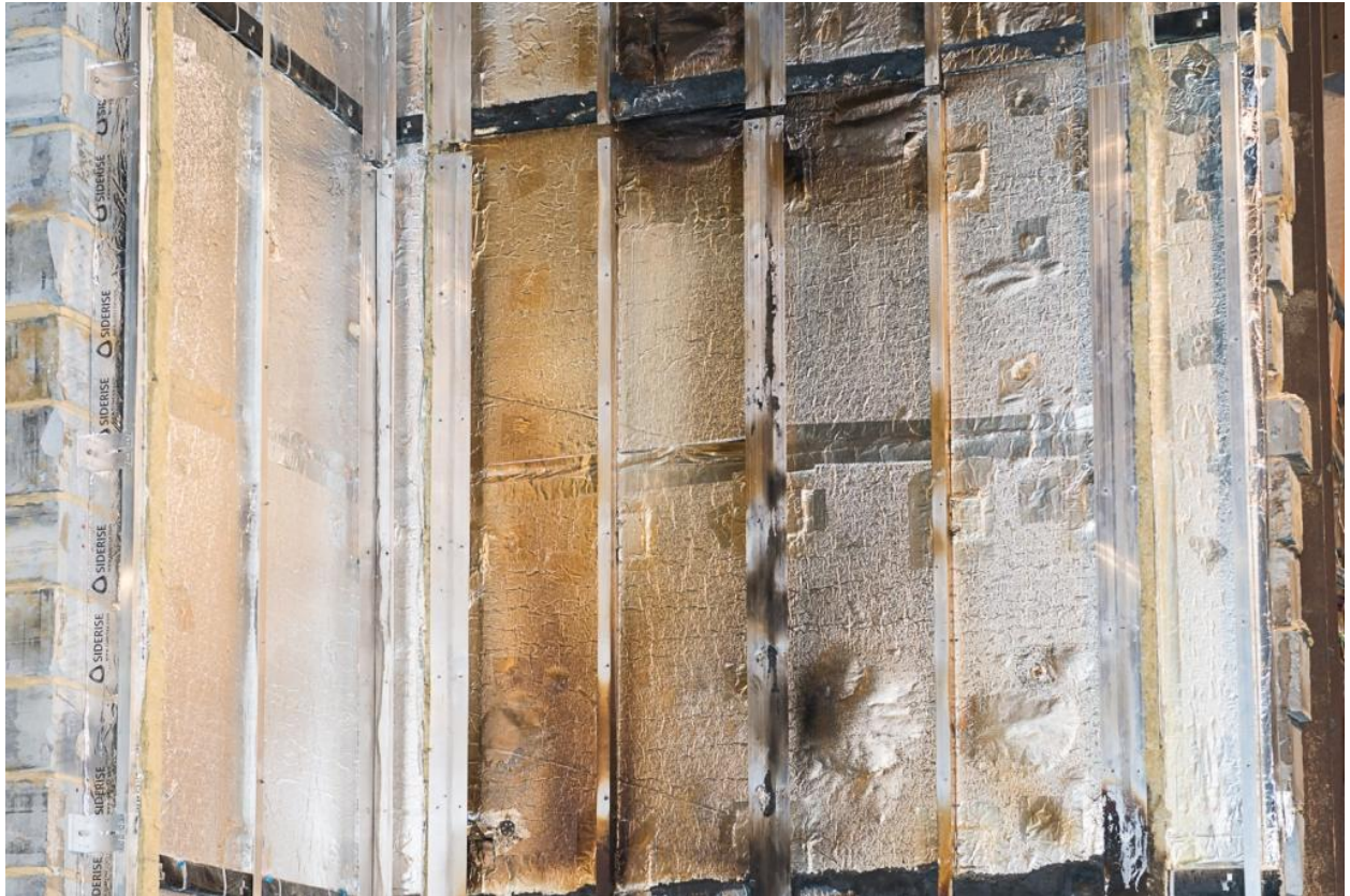
Figure 29. Damage to cladding system beneath ACM panels between the second and third horizontal cavity barrier (approximately 2400-4700mm above combustion chamber).
