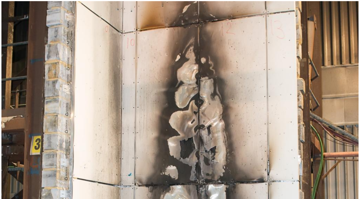
Figure 23. Second row ACM panels (approximately 2300mm-4600mm above combustion chamber).
