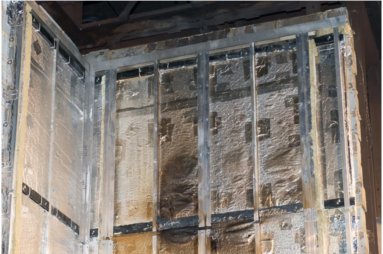
Figure 30. Damage to cladding system beneath ACM panels between the third and fourth horizontal cavity barrier (approximately 4700-6360mm above the combustion chamber).
